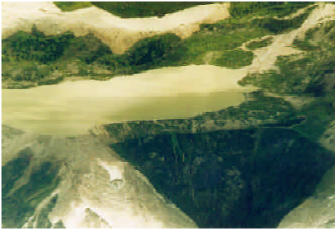
Plate 9.16: Raphstreng Lake, right lateral moraine, glacial snout, the new excavated outlet, and erosion caused by the flood of 1994 along the main river bed.
