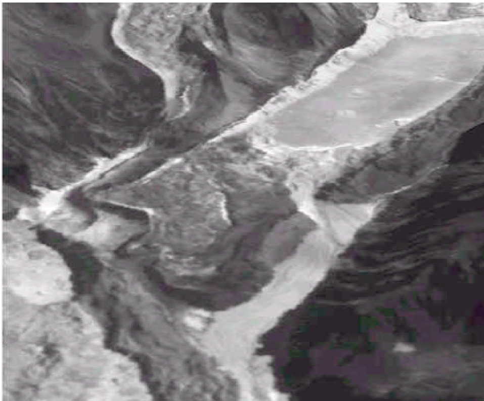
Figure 6.8: IRS1C PAN data of 3 January 1999 draped on the DEM showing the breached area of Luge Tsho Lake on 7 October 1994
